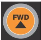
The FWD (Forward) button feeds the Moving Printing Bed in the forward direction (towards the rear of the printer) only as much as the Moving Printing Bed has been fed by using the reverse button. This button also changes a setting in reverse order when selecting settings in Menu mode.
