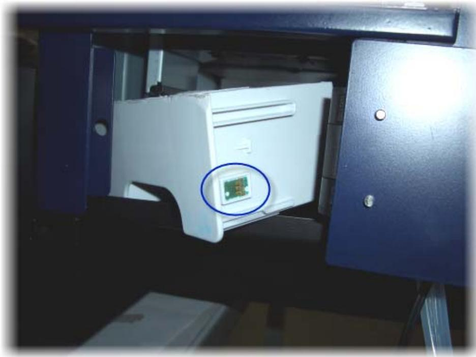
If the following messages / indicators appear on the Control Panel, open the Maintenance Tank Compartment, slide out the Maintenance Tank and apply the Chip Resetter to the ink count chip on the side of the Maintenance Tank as described in Section 0 above. Once the chip has been reset successfully, slide the Maintenance Tank back into the compartment, and close the door:
