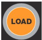
The Load button, when pressed, will move the Moving Printing Bed towards the rear of the printer (Forward) until the Media Sensor is triggered (usually by a platen). Once triggered, the bed will roll towards the front of the printer (Reverse) for a small movement, then forward again until the platen edge is resting against the Media Sensor. These movements are very precise, and if the platen is loaded correctly, provide an accurate and repeatable starting position for the prints.
