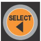
The Select button is used to select a "paper source" ( Roll Auto Cut On /  Roll Auto Cut Off /  Sheet). **Note that this selection should always be Roll Auto Cut Off for normal operation of the DTG Viper™.** It also returns to the previous level menu when pressed in Menu mode.
