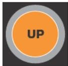
The UP button, when pressed, will raise the Moving Printing Bed (and therefore any media that is positioned on it) until the button is released, the upper limit is reached OR until the Gap Sensor Beam is triggered (which will automatically stop the upward movement of the Moving Printing Bed).
