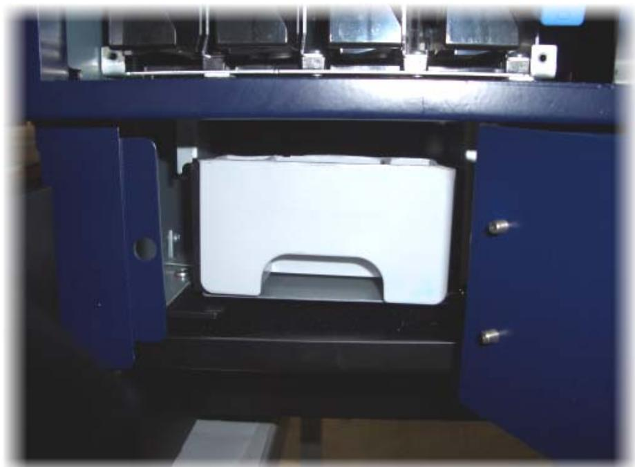
As with the ink count chip on the Cartridges, the Chip Resetter can be used to reset the Maintenance Tank ink count chip.
