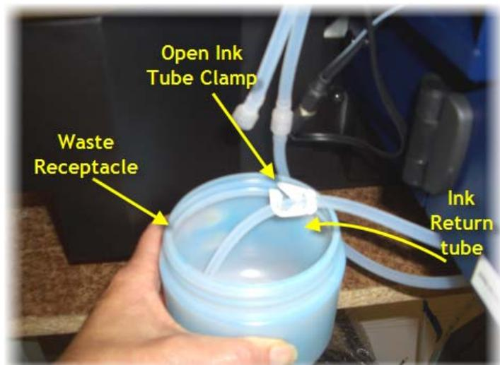
Switch on the mains power to the printer (do not press the Power button on the Control Panel), and connect the power socket for the WIMS unit to start the pump that circulates the White Ink through the WIMS.
