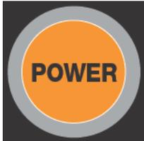
The Power button turns the Printing Head Unit on or off. Note that the main A/c power to the base unit must be connected to the A/C Power Port and switched on at the A/C Power Switch in order for this button, and in fact most functions of the Control Panel to be operable.
